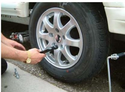
Using the AL-KO combi wheel brace or wheel spanner, remove the wheel bolts and the wheel to be changed.
