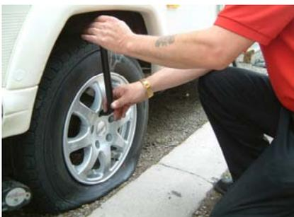
Using the AL-KO combi wheel brace, or AL-KO wheel spanner, slacken off (but DO NOT remove completely) the wheel bolts on the wheel to be changed.
