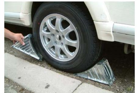
Remove the AL-KO wheel chocks from their carrier fixed to the underside of the caravan floor, and chock the wheel on the opposite side of the one to be changed.
