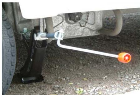
Position the AL-KO side-lift jack into the jack brackets. Raise AL-KO side-lift jack sufficiently to allow the wheel to be removed, and the replacement wheel to be fitted.
