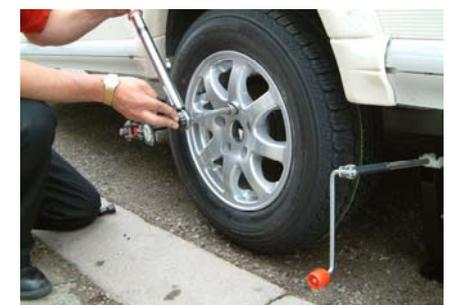
Locate the replacement wheel onto the brake drum and fasten wheel bolts finger tight. Using a torque wrench, torque up the wheel bolts to the manufacturer's recommended setting in the correct sequence i.e. North, South, East and West. Remove the axles stand (if used), raise the corner steadies, raise jockey wheel and release the handbrake.
