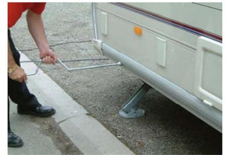
Use the AL-KO corner steady brace to lower the corner steadies on the same side as the wheel to be changed. This is to assist stability of the raised caravan. DO NOT use the corner steadies to jack up the caravan. For additional safety we recommend the use of an axle stand, if available.
