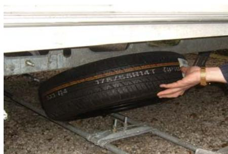
Take out the security chain pin and unfasten the plastic nut of the AL-KO spare wheel carrier. Slide it out to its full extent and remove the replacement wheel. Slide the AL-KO spare wheel carrier back into position and refasten the black plastic nut and security chain pin.
