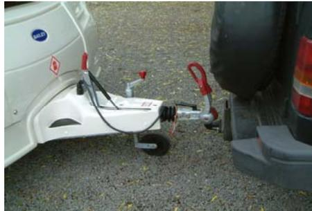
Lower the jockey wheel to the ground and clamp in position. This is to assist with weight distribution when the wheel is lifted.
